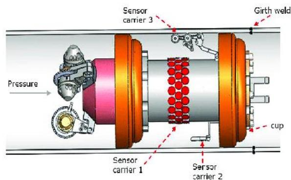
**Figure 4: Pipe Inspection Gauge [26]**
