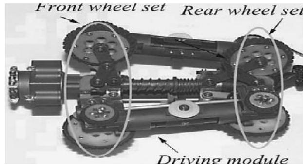
**Figure 5: Wheel Type Inspection Model [38].**
