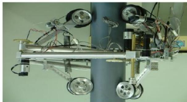
**Figure 3: Spring-Assisted Pipe Inspection Model [2]**
