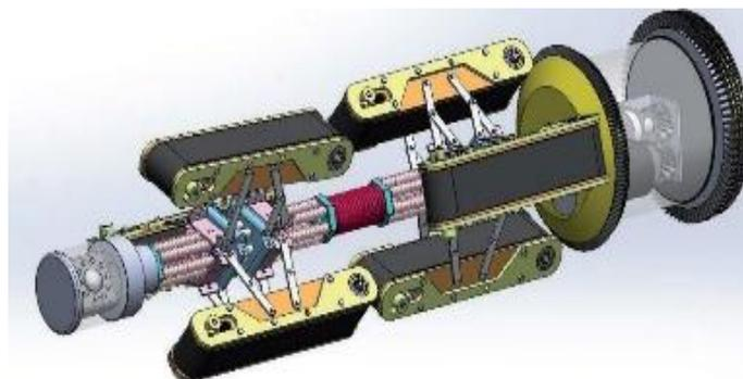
**Figure 6: Track Type Inspection Model [41].**
