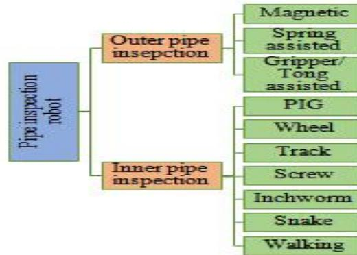
**Figure 1: Classification of Pipe Inspection Robot.**
