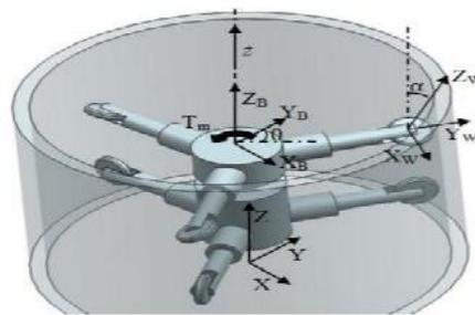
**Figure 7: Screw Type Inspection Model [52]**
